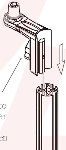
Install to the proper position and fasten
